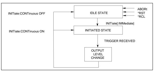
Figure 7-1. Model of Output Trigger System
